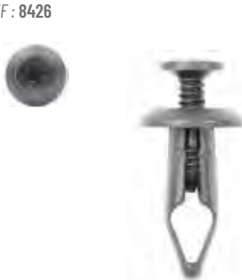
Rivet noir Chrysler/Ford type vis (x50) Head - 15,0 mm • Stem 21,0 mm Hole Size 6,5 mm • OE 6202871 & N8039465 REF : 8189
